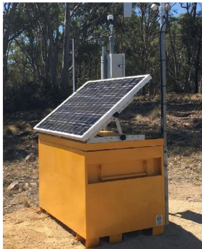
Portable and real-time dust monitor installed at TCM in 2018
